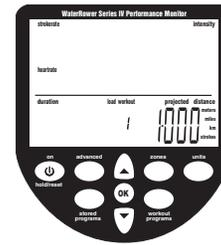
The WaterRower S4 monitor includes an AutoStore function which automatically stores the last 9 historic workout program settings. Programs may be viewed (and selected) using the S4 monitor's AutoPreview function.
